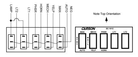
LT1 and LT2 Lighted Rocker Switches may control devices directly bypassing the unit.
